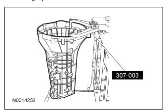
6. Using the special tool, install the manual control lever shaft seal and lubricate it with petroleum jelly.
